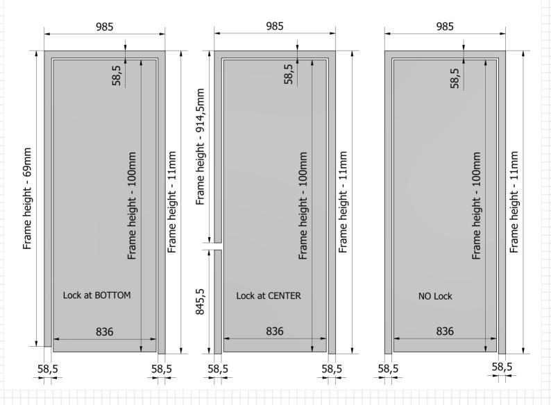
Determine panel dimensions for b62 pivot double door
